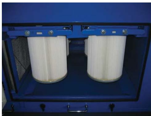
Fasten the Cartridge Clamps. Put on (2) Clamp Fixing Plates and fasten them to the Cartridge Clamp Fixing Base with (4) 5/16" x 3/4" Hex Screw and (4) 5/16" x OD18 x 2t Flat Washers.
